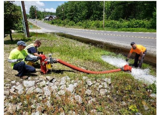
Matt Norris, Dennis Bell and Gary Hebert testing hydrant flow and pressure using the Big Boy Hose Monster, innovative new technology to calculate fire flow ratings from single hydrants.
